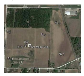
Based on the subsurface conditions encountered and the area geology, the Seismic Site Class is closest to E in accordance with IBC 2009. If soil improvement is utilized and RAP installed, the site classification would be closest to D in accordance with the provisions of IBC 2009.
